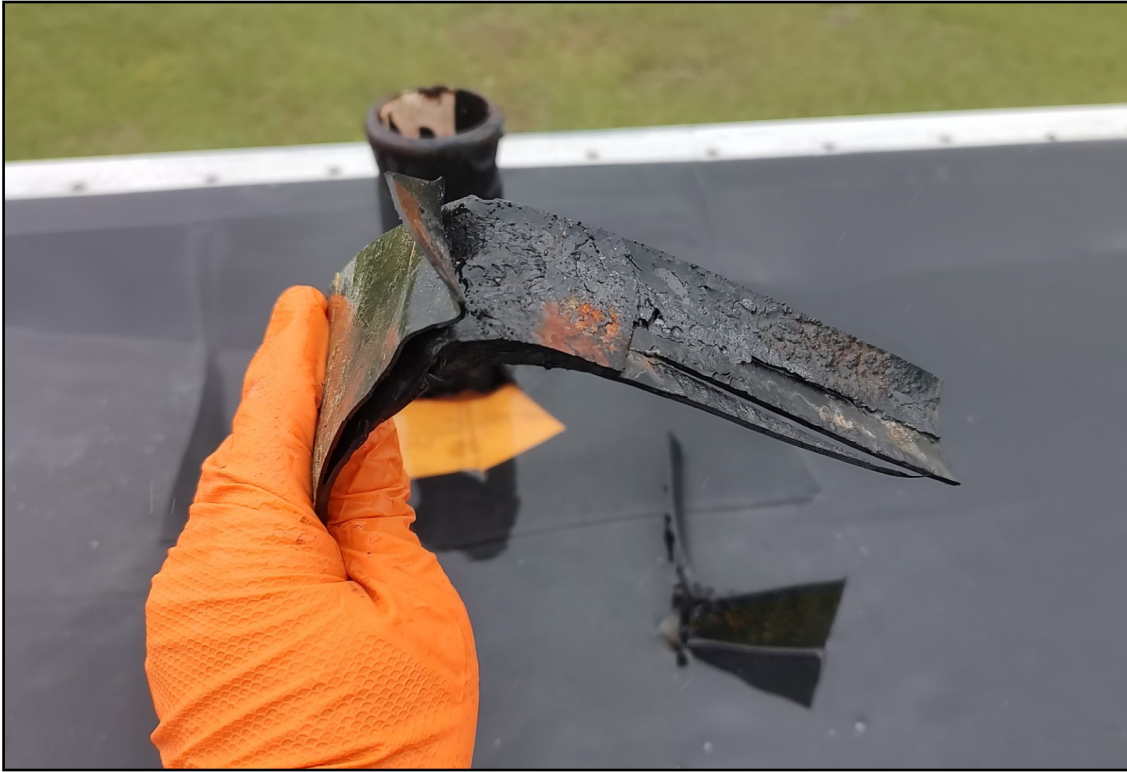
11. View of HA #18—Black Adhesive at Vent Pipe Penetration on the Upper Main Roof at the North Center Area at the Vent Pipe. Laboratory analysis reports this material contains 2% Chrysotile.
