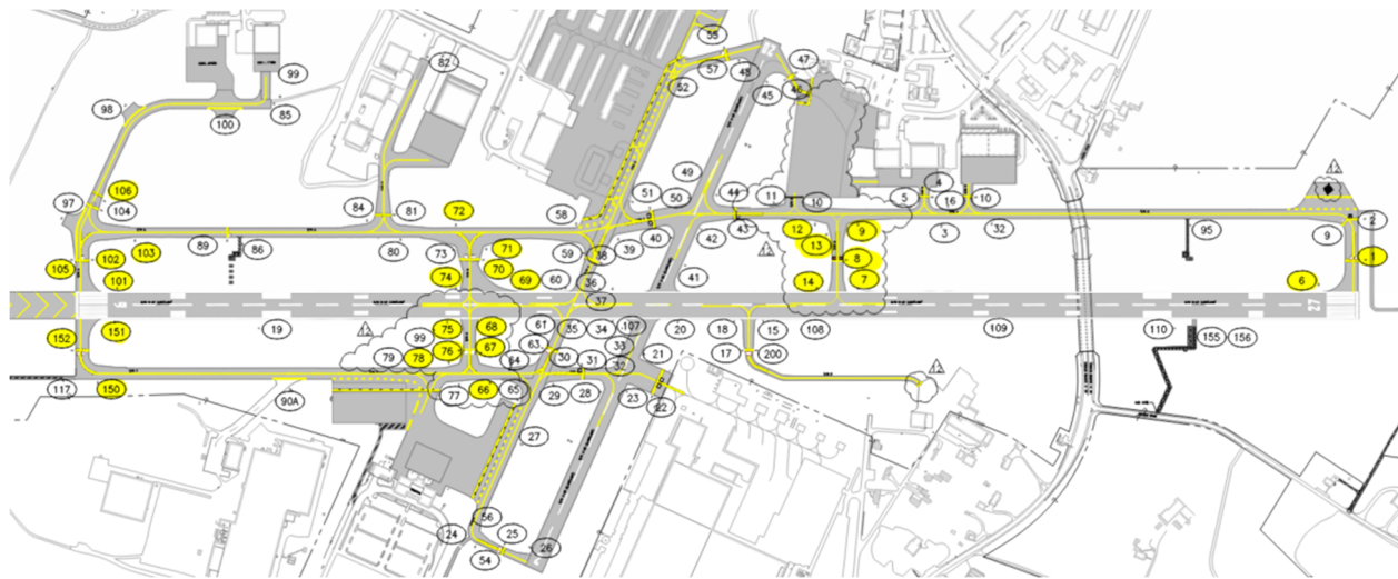
Figure 5.4 –Signs Impacted from Taxiway Name Changes
