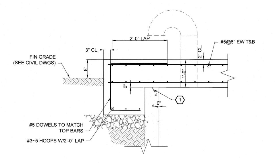
DETAIL - NEW CONC SLAB SCALE: 1" = 1'-0"
