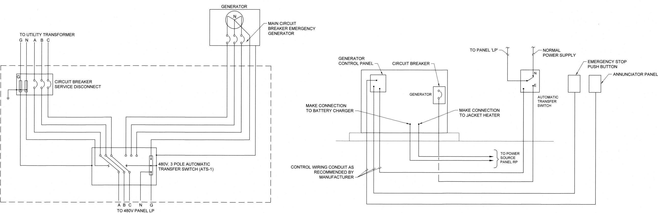
EMERGENCY GENERATOR, ATS AND MAIN CIRCUIT **BREAKER GROUNDING CONNECTION DETAIL** E-601 NOT TO SCALE
