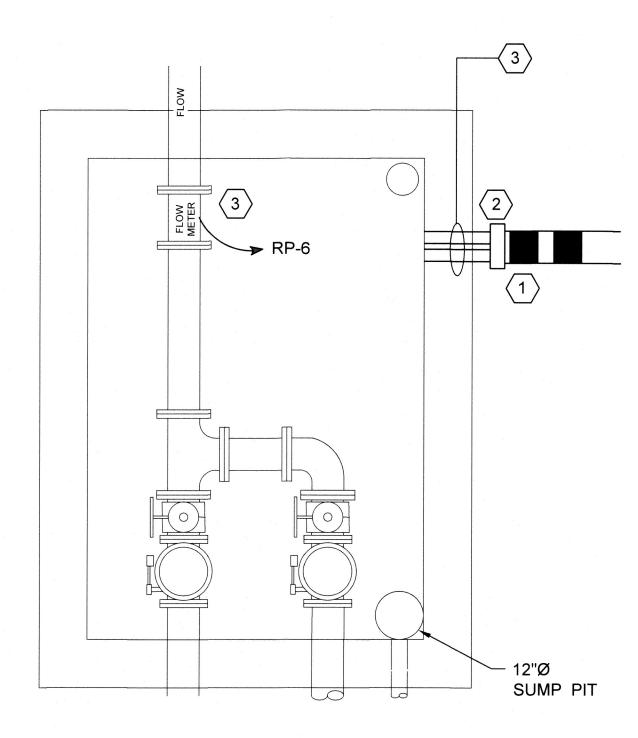
UNDERGROUND VALVE VAULT NEW WORK PLAN SCALE: 1/2" = 1'-0"
