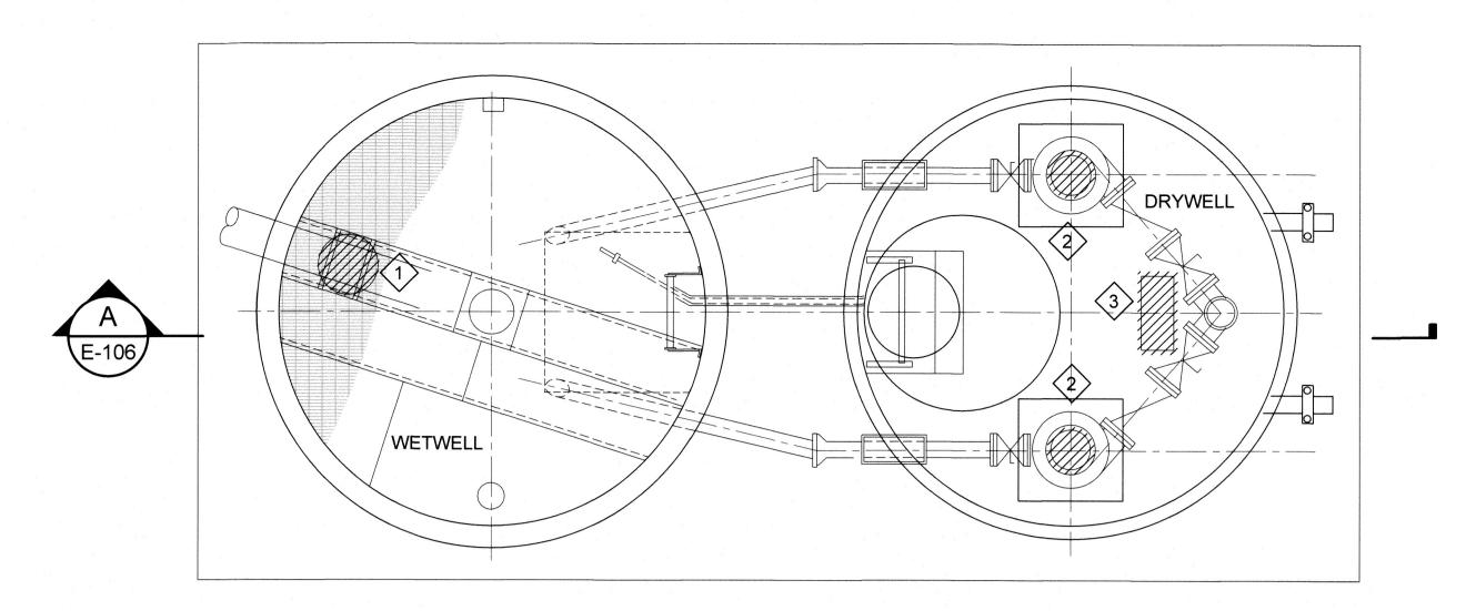
SECTIONAL PLAN PUMP STATION & WET WELL SCALE: 1/2" = 1'-0"
