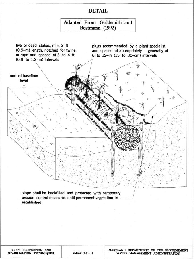
1. DETAIL SHOWN INTENDED FOR CONTRACTOR'S USE IN SLOPE PROTECTION AND STABILIZATION FOR STREAM BED REPAIR AFTER FORCEMAIN INSTALLATION. CONTRACTOR SHALL PROVIDE CONSTRUCTION SUBMITTAL FOR ENGINEERS REVIEW AND APPROVAL PRIOR TO INSTALLATION.
