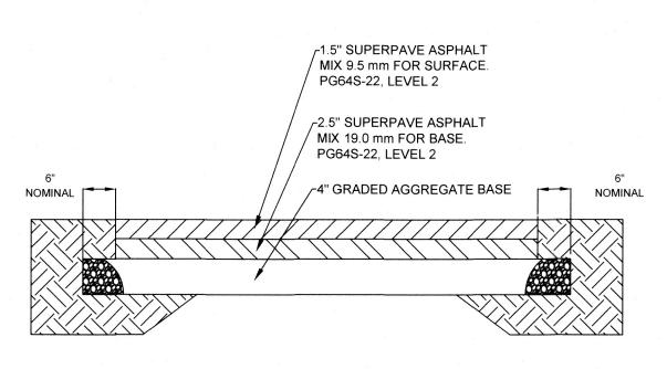
MDSHA 508.08 - DRIVEWAY - FLEXIBLE PAVEMENT SECTION NOT TO SCALE
