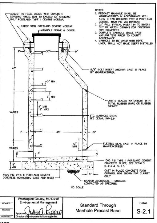
1. REQUIREMENT OF PRE-CAST DESIGN SIGNED AND SEALED BY MD PE WHERE DEPTH EXCEEDS 10 FT. SUBMITTAL FOR PROPOSED MANHOLE TO BE PROVIDED FOR ENGINEER REVIEW AND APPROVAL PRIOR TO INSTALLATION.
