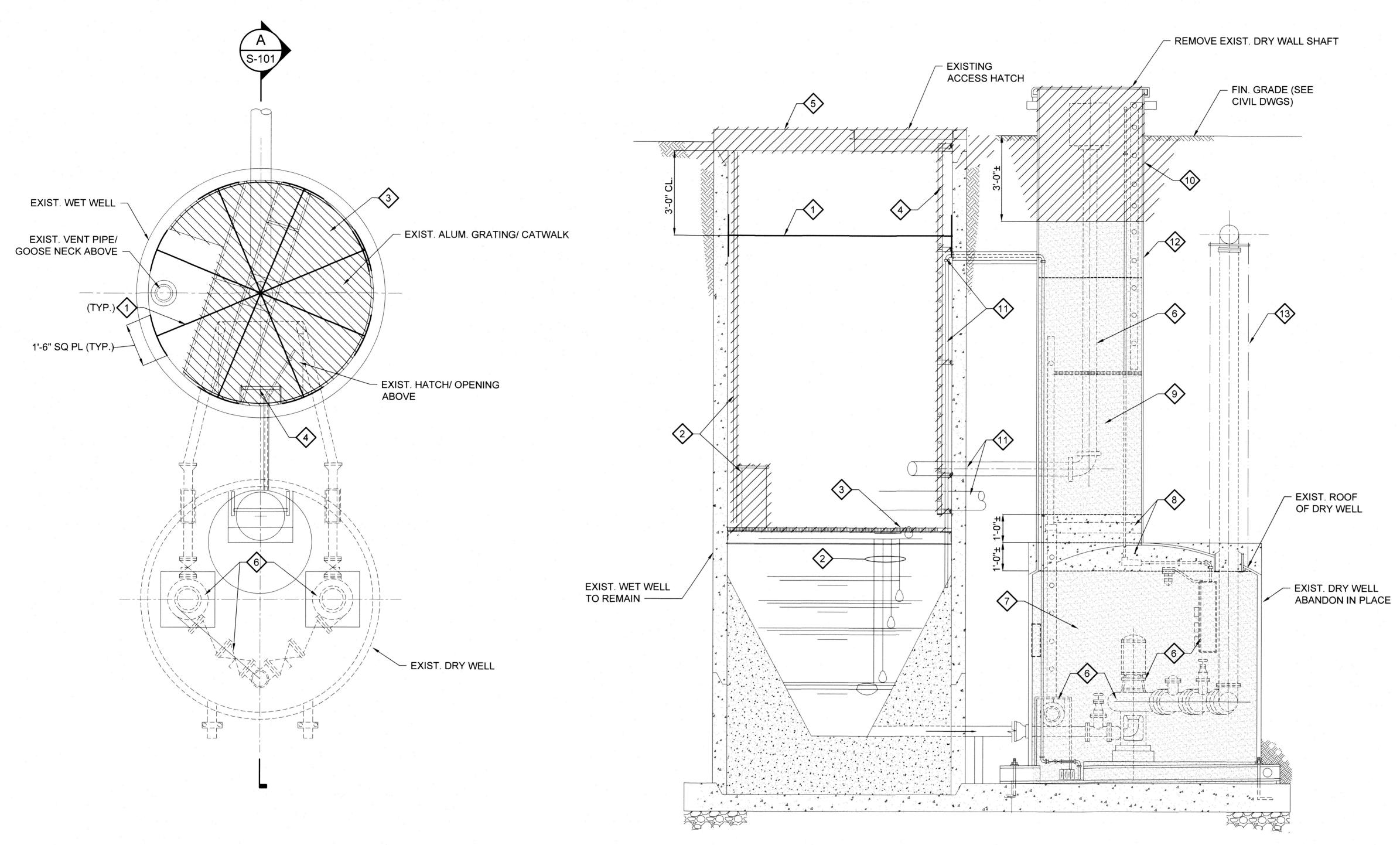
WET WELL AND DRY WELL DEMOLITION PLANS
