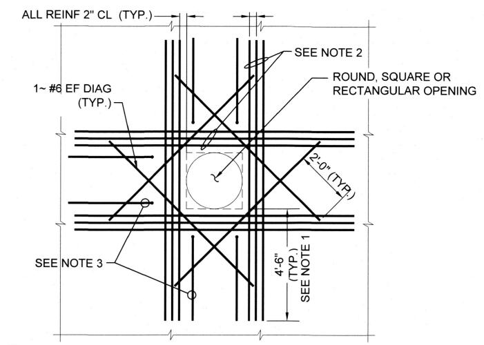
**TYP. ADDNL REINF AROUND OPENINGS** NOT TO SCALE
