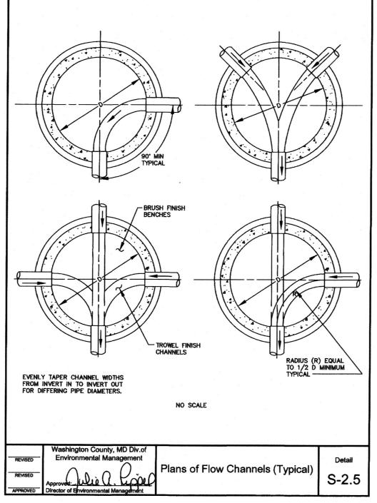
AT TRANSITION MANHOLE FROM FORCE MAIN TO GRAVITY, PROVIDE SMOOTH UPWARD SLOPING CHANNEL FROM FORCE MAIN TO GRAVITY SEWER
