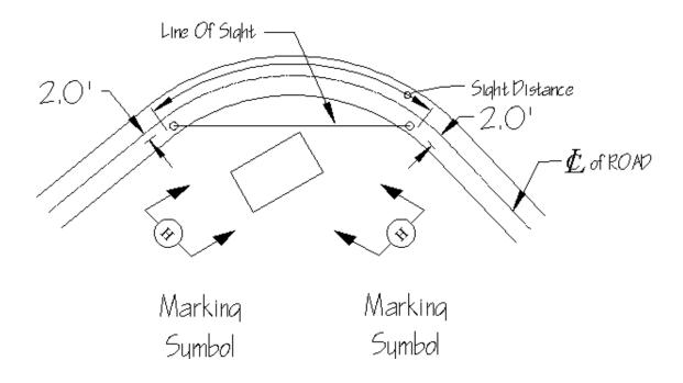
**FIGURE A-2** – Horizontal Curve Sight Distance Measurements
