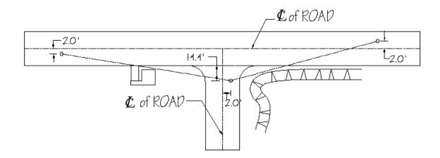
FIGURE A-4 - Intersection Sight Distance Measurements
