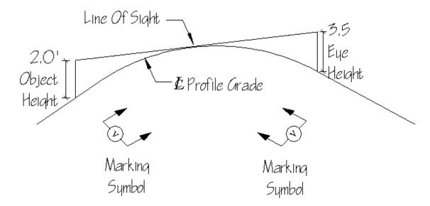
FIGURE A-3 – Sight Distance Measurement on a Vertical Curve
