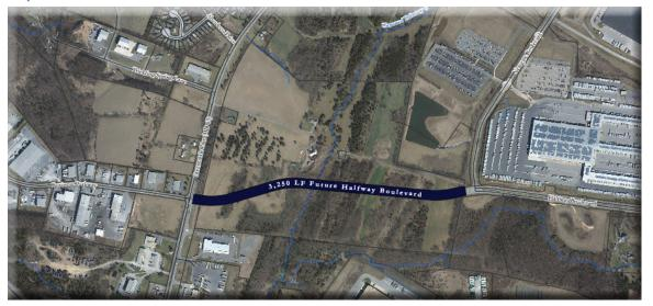
The project involves the construction of 3,250 LF of a four-lane open-section road and major culvert to connect MD Route 63 (Greencastle Pike) to existing Halfway Boulevard at Newgate Boulevard. The extension of the road will facilitate commercial development of the surrounding land and accommodate heavy truck traffic in the area by providing an alternate route between Interstate 81 and Interstate 70.
