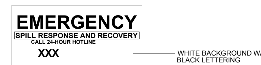
SIGN DIMENSIONS: 8" WIDE X 4" HIGH EMERGENCY RESPONSE - SIGN #4 9 SCALE: N.T.S. S-7
